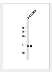
Anti-SNRPD3 Antibody (N-term) at 1:2000 dilution + COLO 205 whole cell lysate Lysates/proteins at 20  $\mu$ g per lane. Secondary Goat Anti-Rabbit IgG, (H+L), Peroxidase conjugated at 1/10000 dilution. Predicted band size : 14 kDa Blocking/Dilution buffer: 5% NFDM/TBST.
